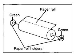
Fix the paper roll holders on both sides of the recording paper roll.
