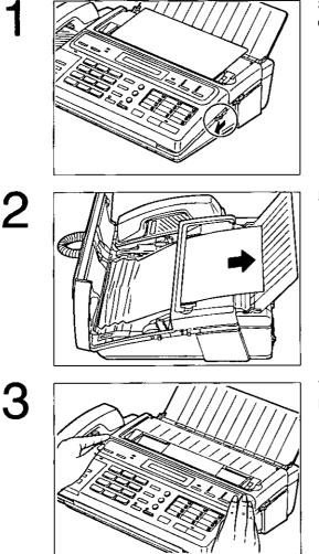
Slide the FRONT LID OPEN lever forward to open the document feeder unit.
