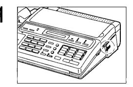
Slide the BACK LID OPEN lever forward to open the paper compartment cover.
